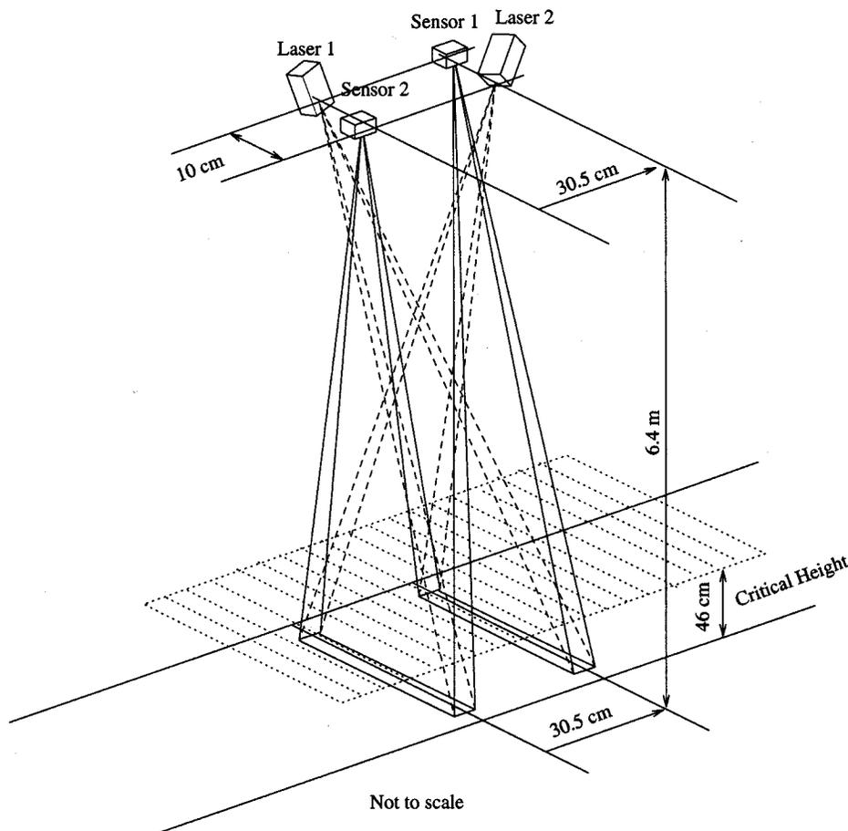
Fig. 3. System hardware configuration.
