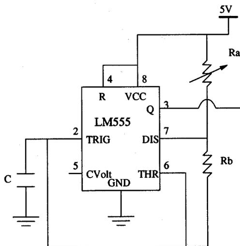
Fig. 9. Clock circuit.
