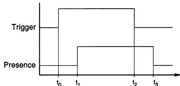
Fig. 16. The timing diagram when a vehicle passes under two sensors.
