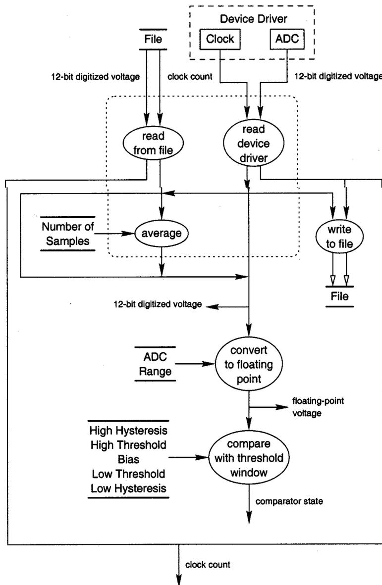
Fig. 14. Functional diagram of the sensor software library.
